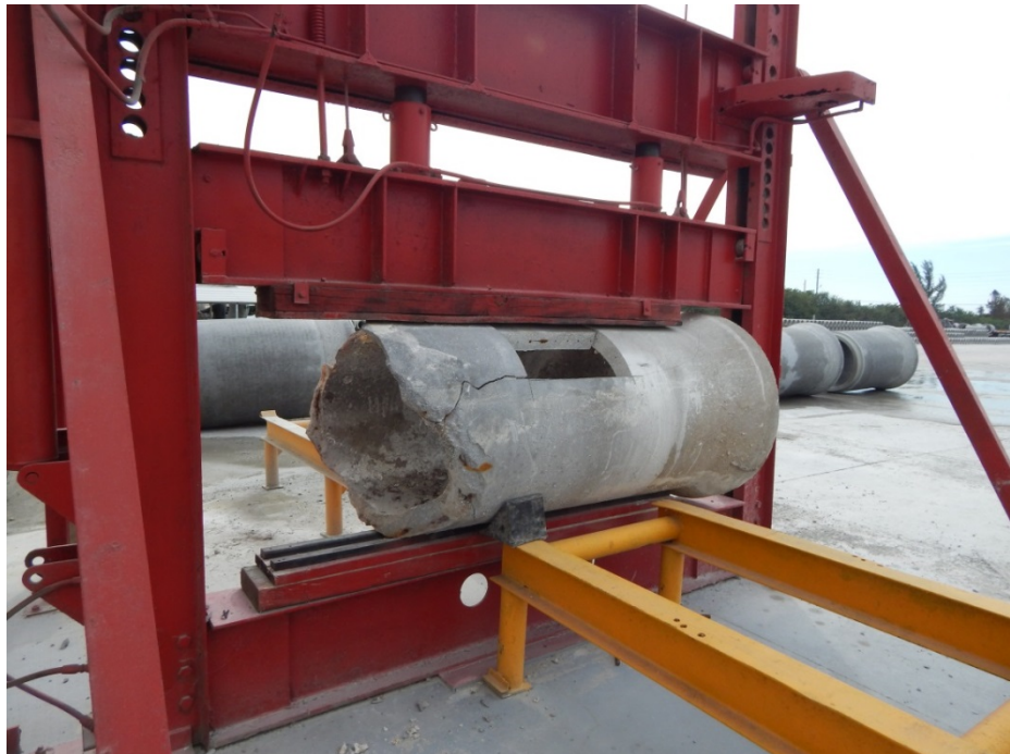
Figure 3. A three-edge bearing (3EB) strength load test was conducted on a 30-year old section of RCP that had been removed from a tidal marina. Prior to loading, a section was removed from the wall for examination. Despite this, the RCP was able to support 51,600 pounds. .
